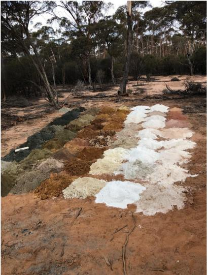
Figure 2. Displaying RC drilling samples
