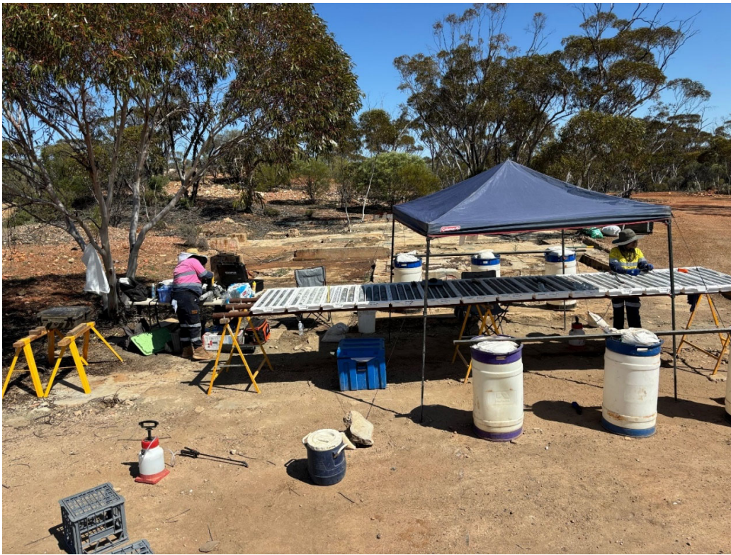
Figure 2: Mt Palmer Gold Mine recent diamond drilling programme – orientation, logging and preparation for assaying by Kula Team.
